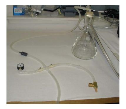
**Figure 5. Tubing Connections of Millipore's vacuum apparatus**. The pressure regulator, vacuum gauge, shutoff valve and pump are connected using 0.25" inner diameter tubing and quick-connect fittings.
