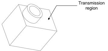
Figure 2. Bio-Cell<sup>™</sup> with approximate orientation for filling. Note that the port opening is tilted upward so that the Bio-Cell can be completely filled.
