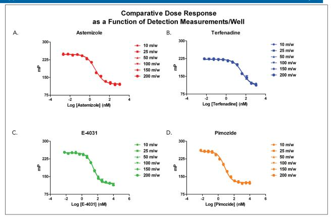
*Figure 7.* Comparative dose response data of 4 known hERG channel blockers for a variety of measurements/well shows high correlation within each compound regardless of detection setting. Table 1 shows comparative  $IC_{so}$  data for each compound.
