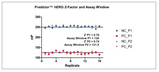
*Figure 6.* Run 2 assay window and Z' results at 2 hour incubation and 10 m/w with a read time of 1 minute 17 seconds for each of 2 plates of data. Values of 111-153 are an expected range for assay windows calculated at incubation times of 1-4 hours, with corresponding Z' values of 0.56 - 0.77 respectively. Z' factors were calculated using the method of Zhang *et al.* (1999).
