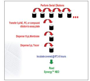
*Figure 4.* Instrument Performance Validation Workflow for Predictor™ hERG Fluorescence Polarization Assay on Synergy™ Neo.
